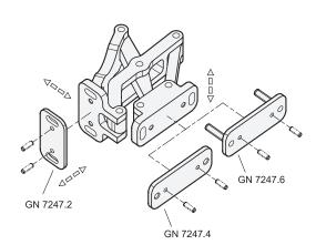
The multiple-joint hinges can be adjusted in three planes during installation. For example, this allows adjustment for tolerances or establishing of required compressive forces for seals.
